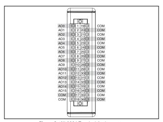
Figure 2. NI 9264 Terminal Assignments
